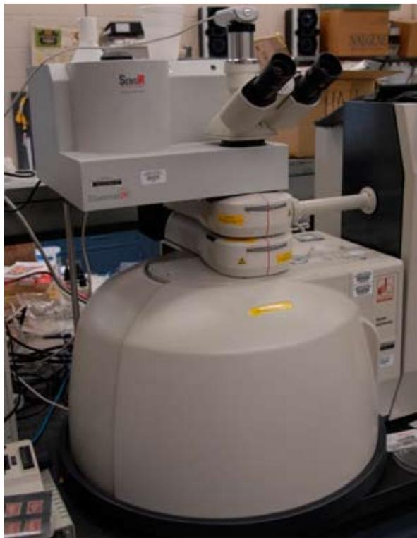
**Figure 7.** The Raman microscope.
