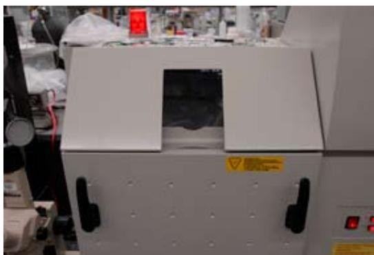
**Figure 4.** The vacuum chamber of the EDXRF spectrometer.
